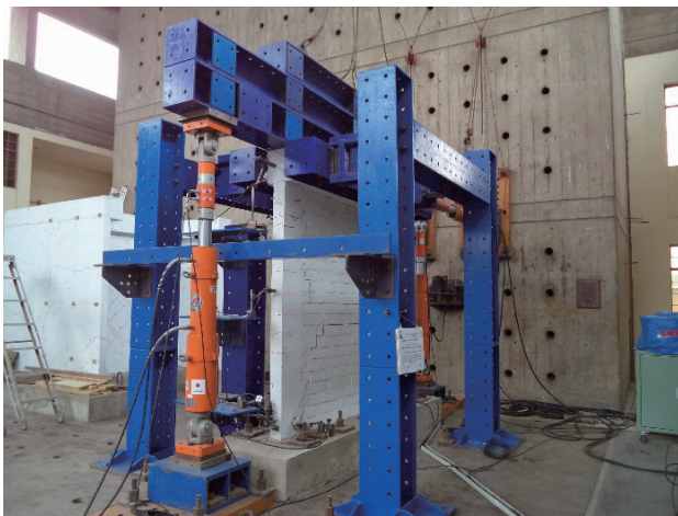
Fig. 7. Test setup for masonry wall test.
