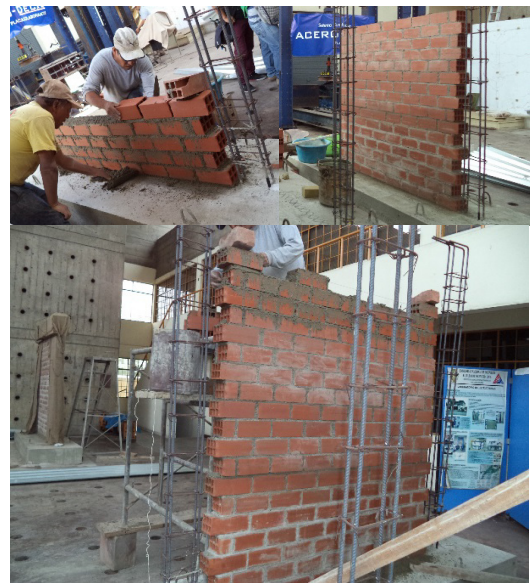
Fig. 4. Three stages of specimen construction.
