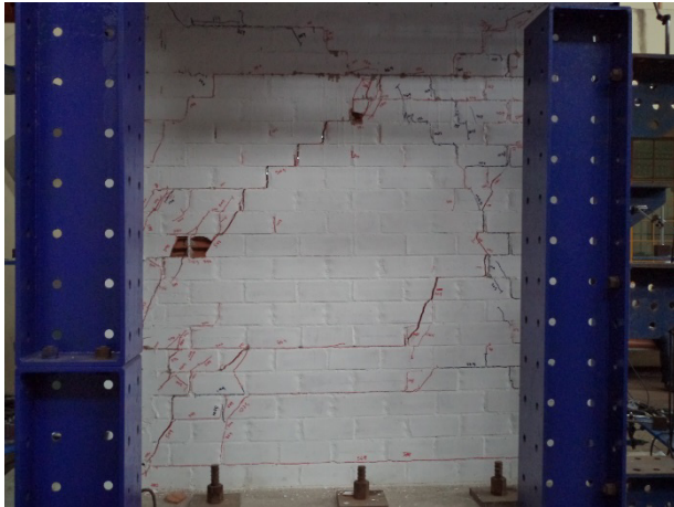
Fig. 9. Final state of wall (1/150) – WALL-SP-1.
