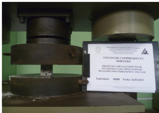
Fig. 6. Compression test of mortar.
