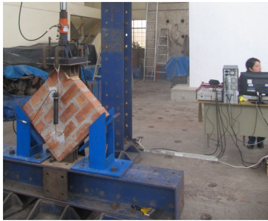
Fig. 14. Diagonal tension tests.
