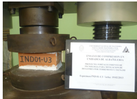
Fig. 4. Compression test of bricks.
