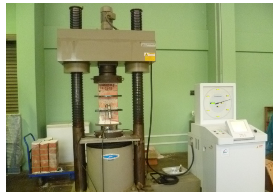
Fig. 8. Compressive strength tests.
