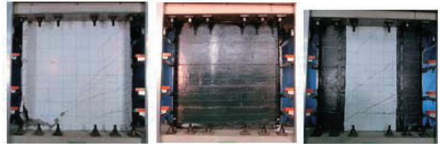
(a) No retrofit (b) Full retrofit (c) Partial retrofit
