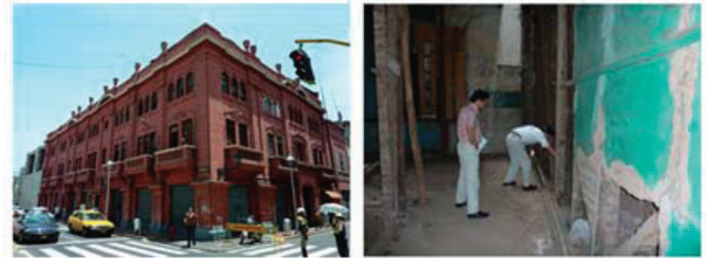
Fig. 10. Microtremor measurement of an adobe building.
