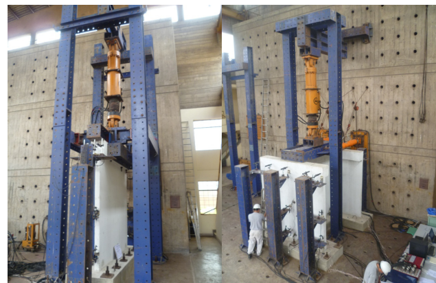
Fig. 15. Test set up for one plane wall and H-shaped wall.
