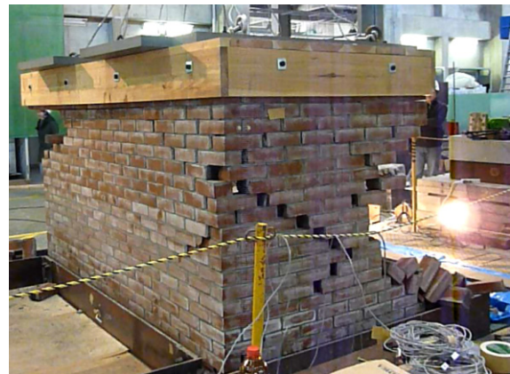
Fig. 13. Shape of failure of the 2 nd specimen.
