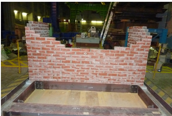
Fig. 10. Shape of failure of the 1 st specimen.
