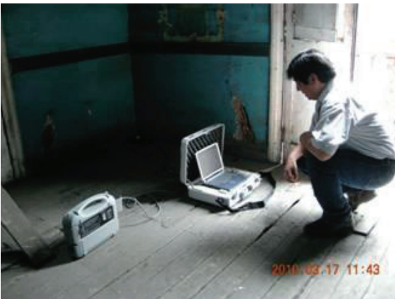
Fig. 9. Microtremor measurement of adobe-quincha building.
