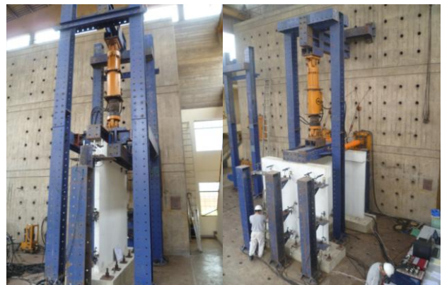
Figure 4: Test Setup on Plane and H walls.
