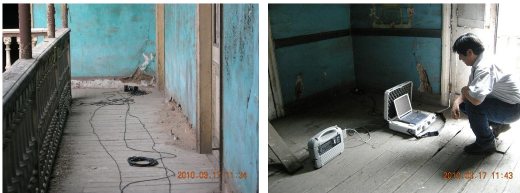
Figure 8. Ambient vibration measurements on adobe-quincha building at historic centre of Lima
