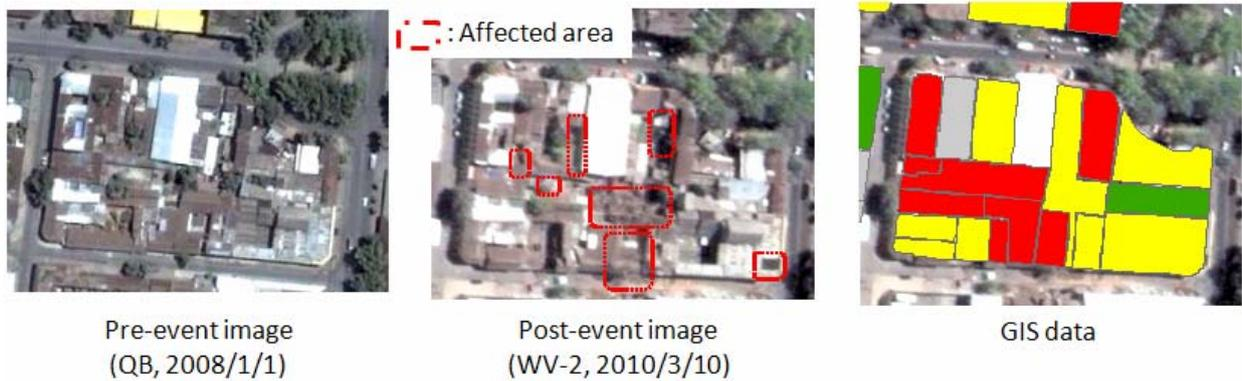
**Fig. 7** Comparison between pre- and post-event satellite images to detect affected buildings
