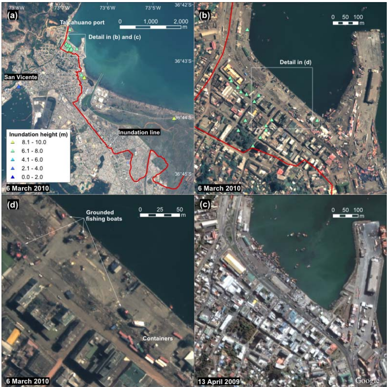
Fig. 5 (a) Result of tsunami height measurement in Talcahuano. The red line indicates the extent of inundation zone which was obtained by the interview with CATOE (Centro de Alertamiento Temprano y Oficina de Emergencia). (b) Damage in Talcahuano found in the post-event satellite image (WorldView-2). (c) Satellite image of Talcahuano before the tsunami attack (13 April 2009, from Google) (d) Close-up view of port of Talcahuano. Grounded fishing boats and drifted containers were seen.
