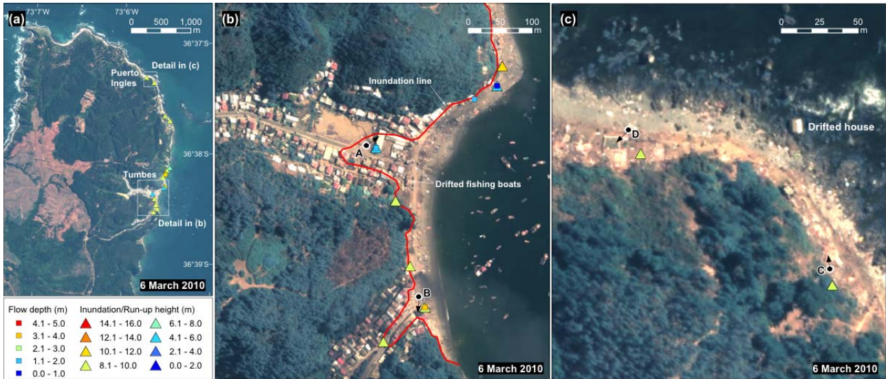
Fig. 10 (a) Overview of tsunami measurements (inundation and run-up heights) in Tumbes and Puerto Ingles. (b) Detailed features of the measurements and the damage in Tumbes. (c) Devastated damage in Puerto Ingles. Point A to D is the position of ground photos in Fig. 11 respectively with the arrow of focus direction.
