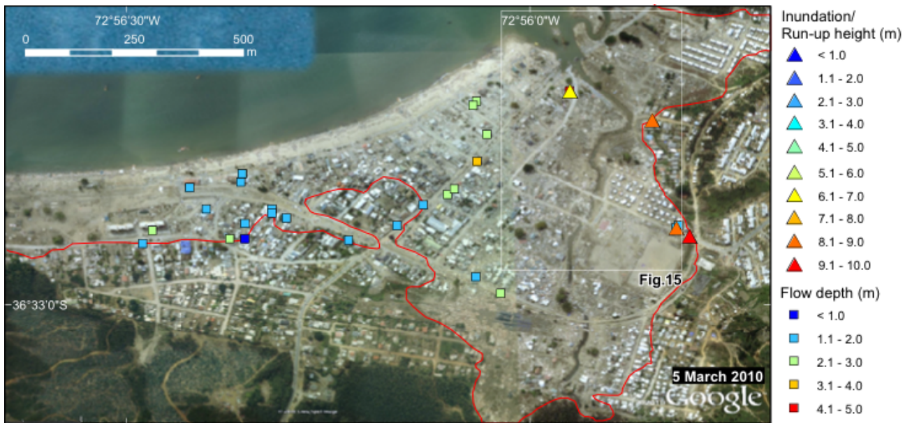
Fig. 14 Tsunami height, flow depth and extent of inundation in Dichato.
