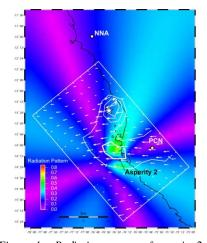
Radiation pattern of asperity 2 (thick white Figure 4. line), 2007/08/15 Pisco earthquake.
