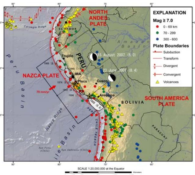
Fig. 2: Tectonic setting and the epicenters of earthquakes in Peru and the surrounding region (modified from [2] and [3])
