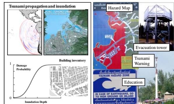
Fig. 6: Tsunami simulation, damage assessment (left) and countermeasures (right)
