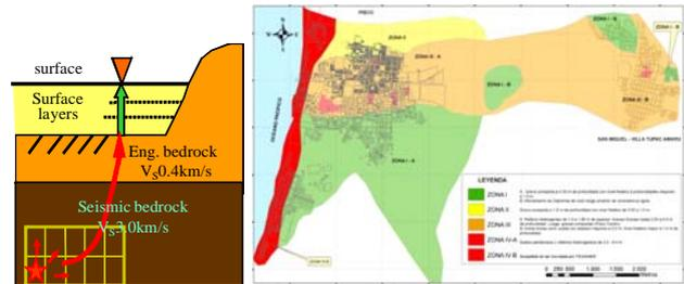
Fig. 5: Simulation of seismic motion (left) and an example of seismic microzonation (right)
