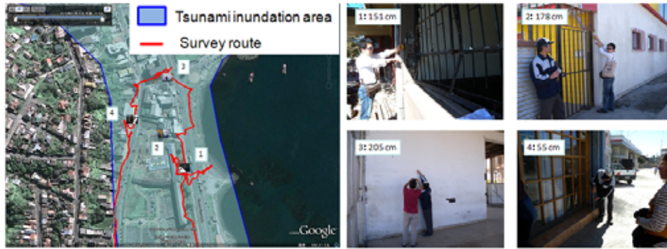
Fig. 10: Measurement of tsunami inundation depth in Talcahuano
