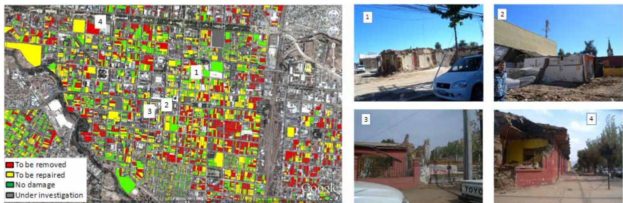
Fig. 5: GIS file to show the damage levels of buildings in Talca and locations of field photos
