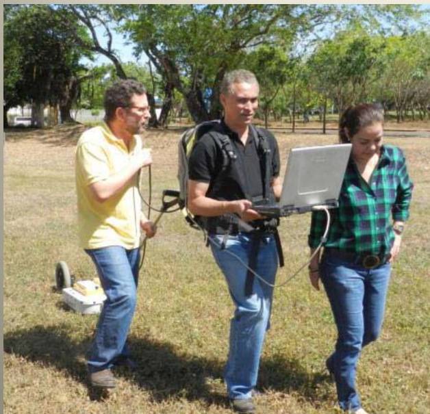
Georadar (GPR-Ground Penetration Radar)
