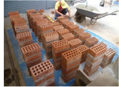
Direct shear specimen
