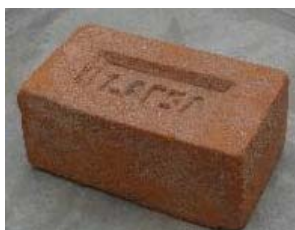
Solid brick (Handmade)
