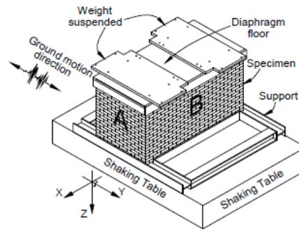
(a) Scheme of the test set up
