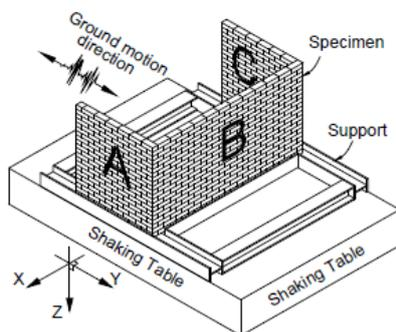
(a) Scheme of the test set up
