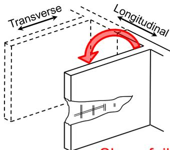
Shear failure of wall ... studied well
