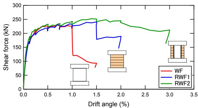
It is confirmed that ductility improve due to wrapping carbon fiber sheet.
