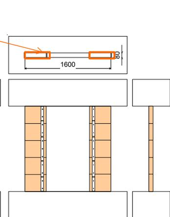
Wrapping CF sheet at the **end of wall** with steel plate and bolt
