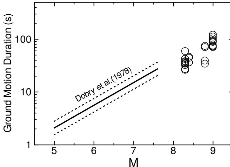
Fig. 11 Relationship between Ground Motion Duration and Earthquake Magnitude
