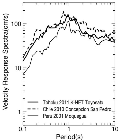
Fig. 9 Comparison of Response Spectra at Stiff Soil Sites from Three Earthquakes
