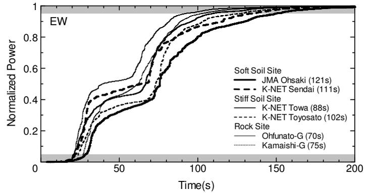
Fig. 7 Comparison of Ground Motion Duration
