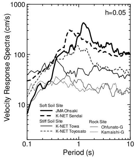
Fig. 5 Comparison of Response Spectra with Different Site Conditions
