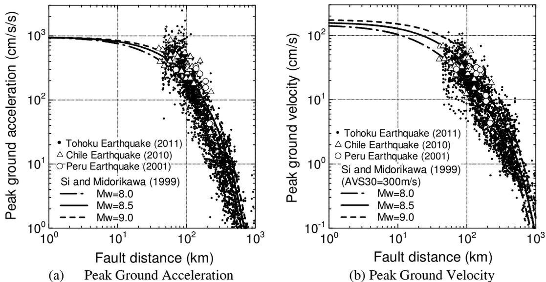
Fig. 8 Comparison of Attenuations between the Tohoku, Chile and Peru Earthquakes
