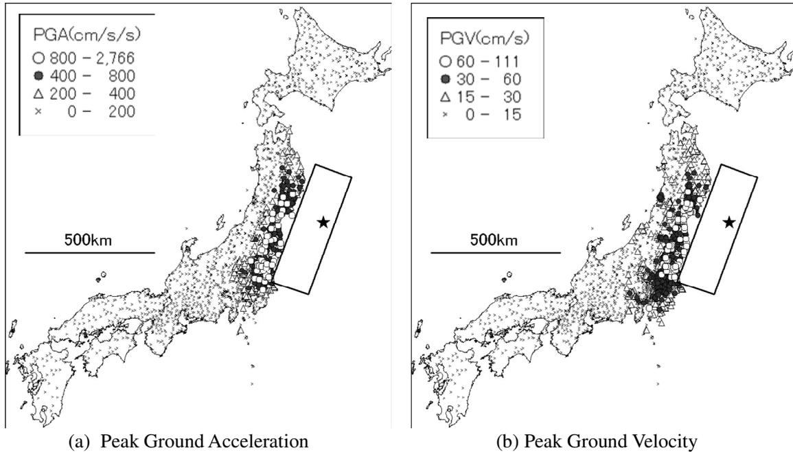
Figs. 2 Peak Ground Acceleration and Velocity of Observed Strong Motion Records
