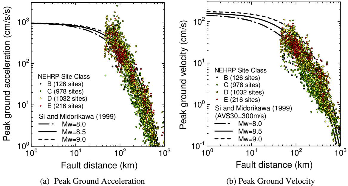
Figs. 3 Attenuation of Peak Ground Acceleration and Velocity
