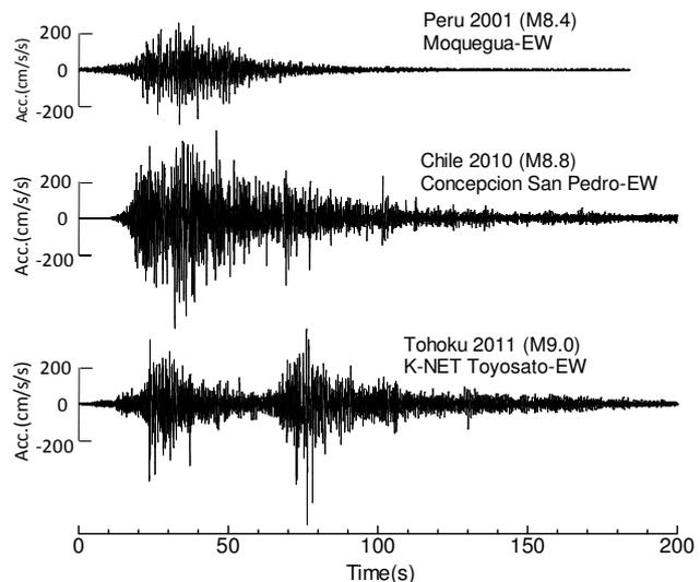
Fig. 10 Comparison of Time Hitories of Records from Three Earthquakes
