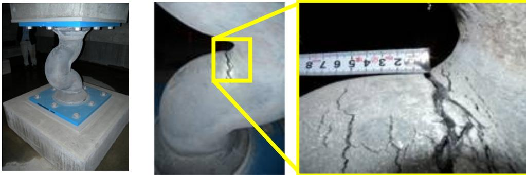
**Figure 8.** Cracks in lead dampers
