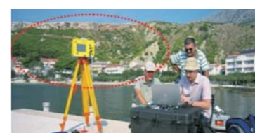
Use of a 3D laser scanner to measure the location of rock blocks with a high risk of collapse that are scattered across the steep slopes of the Adriatic coast (example of measurements made in Duće, on the outskirts of Split)
