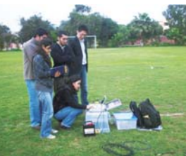
Observations of microtremors in Lima, using equipment provided in this project. This makes it possible to assess ground shaking in the event of an earthquake.
