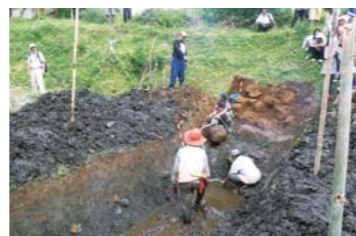
A study of the Lembong fault on the outskirts of Bandung. A trench was excavated at the base of the fault escarpment at the rear. The study of the geological layers revealed that an earthquake had occurred several thousand years ago.
