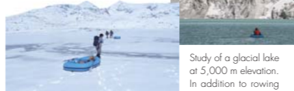
Study of a glacial lake at 5,000 m elevation. In addition to rowing out in a rubber dinghy to measure the water depth, the researchers checked for factors that cause lake outburst, studied the strength of the moraine and so on.
