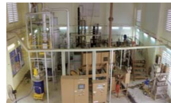
The biomass plant installed on the grounds of Ho Chi Minh City University of Technology to test technology for the locally self-sufficient production of bioethanol from rice straw
