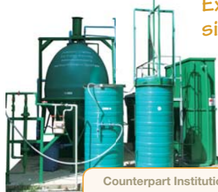
Demonstration plant set up at Chulalongkorn University to conduct test production of recycled water and biogas from campus wastewater and food wastes
